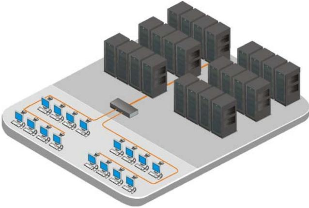
**Cables...** All cabling to the user stations and computers uses standard CATx cable. Max cumulative cable length of 1,000'
