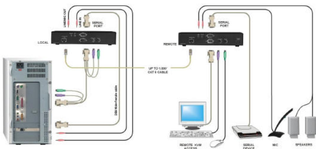
**Figure 1. Typical Installation**
